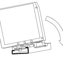
To install the ICM4 on a "T" style rail, angle the module so that the top groove of the "foot" is located over the lip of the top rail. Push the module toward the rail until it snaps into place. To remove a module from the rail, insert a screwdriver into the slot on the bottom of the "foot", and pry upwards on the module until it releases from the rail.
